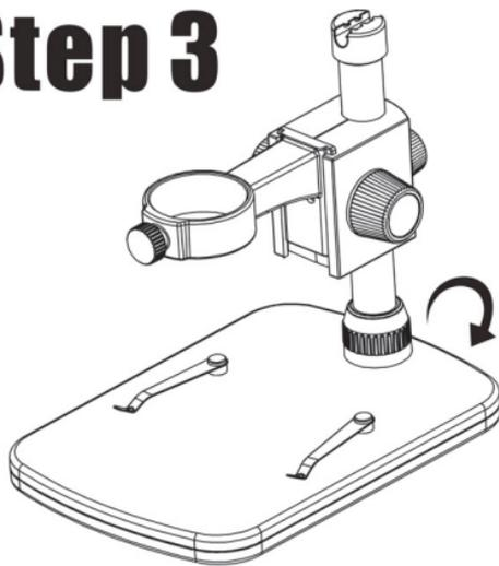
Rotate Screw-7 to fix the pole on the stage.
